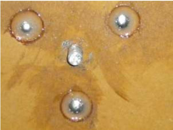
Now get the Drum Disk that has been drying and drill holes for the Bearing Support Bracket (Item #32) Centered around the 3/8" Bolt already installed in the disk. Make sure to Countersink the heads of the 1/4" Carriage Bolts (Item #20) on the side that the 3/8" carriage bolt is protruding from. See photo. Epoxy these bolts in as you did the 3/8" carriage bolt.
