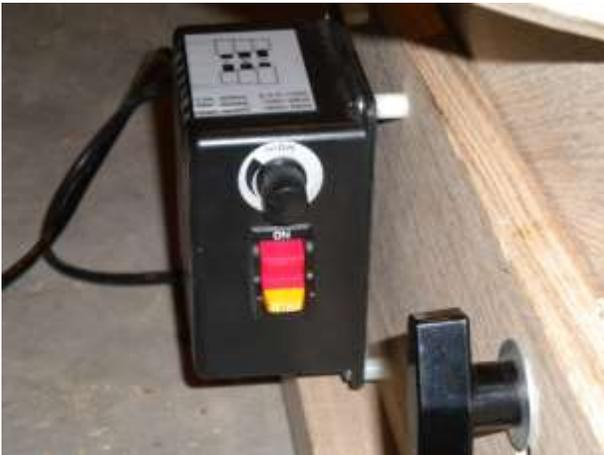
Next install your speed control to the side support using the nylon spacers to keep it set off from the side support. There is a grounding screw that sticks out of the speed control which makes the spacers necessary. They don't need to be as long, but it is what I had on hand.
