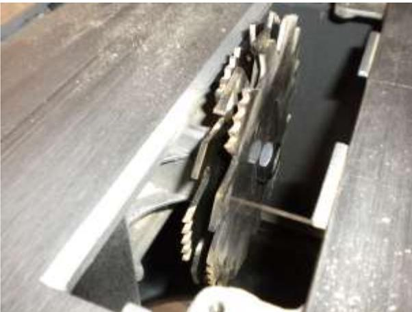
The photo to the left shows the set up of the stacked dado blades. I had to make two passes to complete each groove in the base since my table saw would not accept enough cutting blades. I marked the base and the rip fence so that I had a reference line as to how far to push the base into the blades so the grooves ended up the same length. Make sure to match the width of the groove to the wood you are using. Not all 3/4" lumber is exactly the specified thickness.
