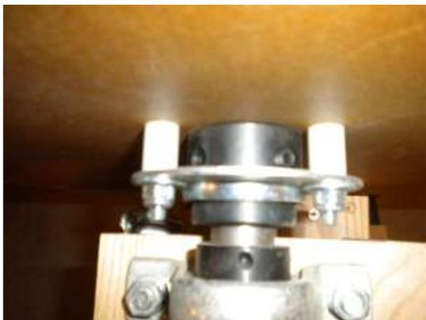
Mount the Drum Disk assembly onto the axle. Tighten the set screw in the step collar securely. Loosen the bearing collar set screws and adjust the Drum Disk so that it does not hit anywhere and the disk is riding on the motor shaft where you would like. Tighten the bearing collars securely at this point.
