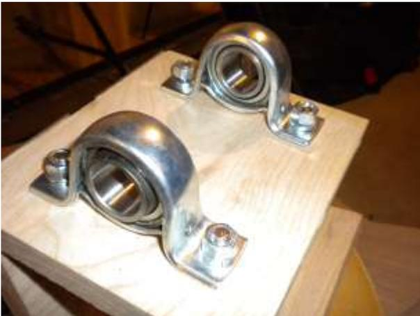
Place the Bearings (Item #31) into the Bearing Brackets making sure that the bearing collar end of both is pointing to the outside and place them onto the carriage bolts. Place a 3/8" Lock Washer (Item #25) and 3/8" Nut (Item #26) onto the carriage bolts, but DO NOT tighten securely at this time.
