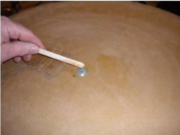
After sanding is complete install the 3/8" x 1 1/2" (Item #17) in a counter sunk hole so the head of the carriage bolt is below the disk surface. Mix and apply enough epoxy to secure the carriage bolt and fill the void remaining above the bolt. Set this aside to dry and continue with making the motor box.
