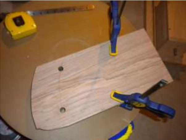
Clamp the two sides firmly together with the scribed line facing up.
