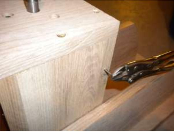
Pre drill a hole in the bottom of the assembled Motor Box to accept a screw with the head cut off. As you can see in the photo a small vise grip pliers was used to turn the screw into the hole. This is done so that you can adjust the screw so it will scribe a mark in the side of the Side Support. This scribed line will be used to cut the slot for the angle adjustment.
