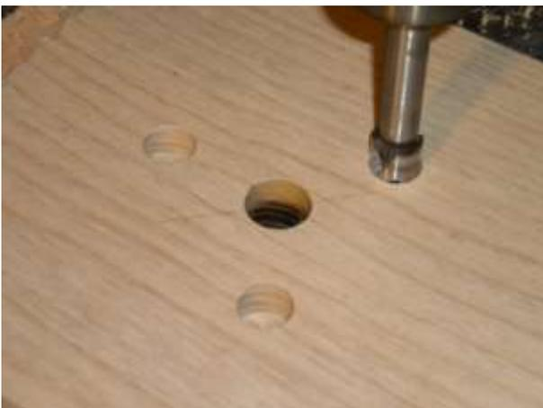
If you are using the recommended motor or one that will mount to the end, layout the hole pattern and drill the holes. Countersink the holes to allow the bolts and washers to be below the surface when tightened. I used a fostner bit to create a nice flat hole. The countersink hole is shown being drilled. The fostner bit will leave a small point in the center of the hole, use that as a reference to drill the bolt hole all the way thru the board.
