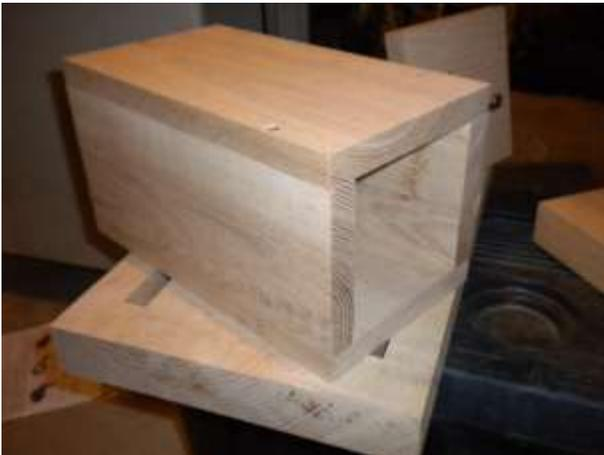
Assemble the Motor Box Top and Bottom (Item #10) and the Motor Box Sides (Item #11). Make sure you are mounting the side pieces inside of the top and bottom. This will form a box that is 6 1/4" square. I did not use glue only screws in case I would have to replace the motor.
