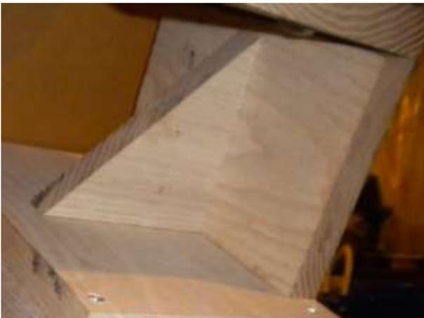
Attach the Drum Support Side Reinforcement (Item #7) to the Drum Support Side, pre drilling and using screws.
