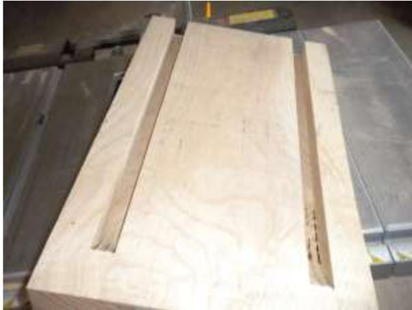
The photo to the left shows the Base (Item #1) with the grooves cut into it. Note that there is material left by the blades at the end of the cut. You will need to make cuts in the Sides to accommodate this or if you have the tools to remove the extra material and want to that is also an option.
