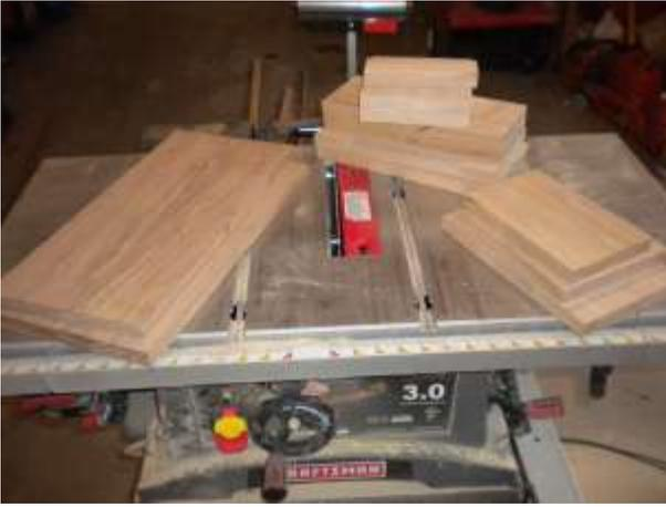
I recommend using a hardwood in the construction. Pre drilling all holes will be necessary. Do not try to over tighten the screws when assembling or the screws may break.
