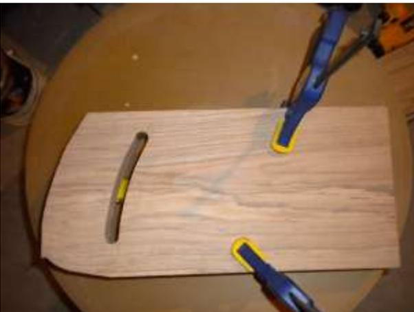
Measure 5/16" on each side of the scribed line at small intervals to make guide lines for cutting the slot. Using a reciprocating saw cut the slot in the Side Supports. You can sand this slot if you like, but it is not necessary.
