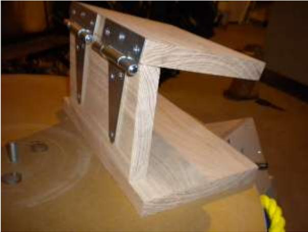
Assemble the Drum Support Bottom (Item #5) to the Drum Support Side (Item #6) pre drilling and using screws.
