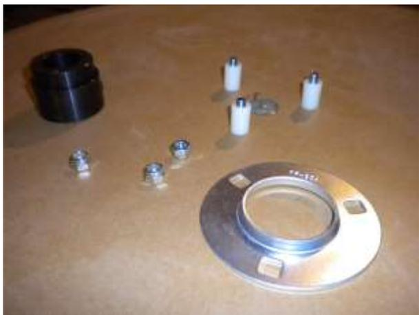
Go find that disk that has been drying and place the Nylon Spacers (Item #22) onto the carriage bolts then a Flat Washer (Item #23). Place the Step Collar (Item #28) over the 3/8" carriage bolt that was epoxied in making sure the small end of the step collar is up. Then place the Circular Bearing Holder (Item #27) over the 1/4" carriage bolts and step collar, then place another Flat Washer and the Lock Nut onto the 1/4" carriage bolts.
