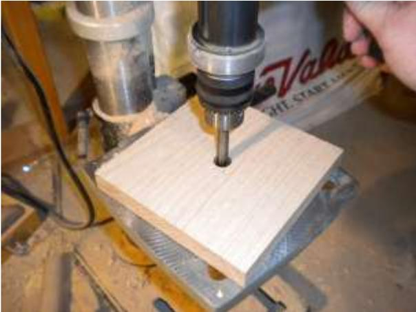
Take one of the Motor Support Ends (Item #9) and drill a hole in the center to accommodate the motor shaft. Make sure it is big enough so the motor shaft does not bind.
