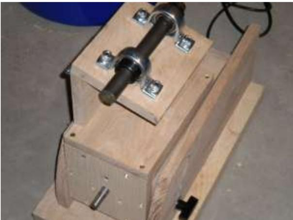
Mount the Drum Support Assembly to the top of the Motor Box Assembly at this time by pre drilling holes and using screws.
