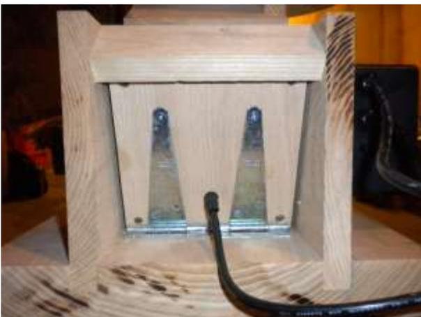
With the Side Supports (Item #2) inserted in the grooves of the Base attach them with a couple screws to affix them temporarily. They will not fit all the way down in front at this point.
