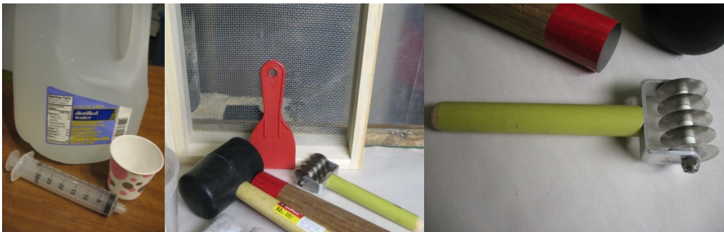
Figure 2 Distilled water, syringe & cup, red plastic putty knife, 8 mesh screen, rubber mallet & wooden ram, special round cutter.
