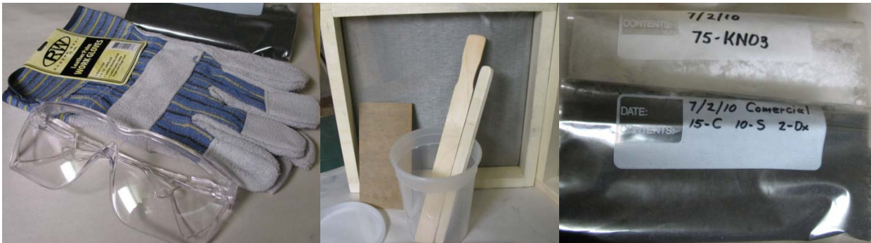
Figure 1 Safety glasses & gloves; 100 mesh screen, mixing container & lid, wooden paddles & plastic laminate; Potassium nitrate (oxidant), Fuel (charcoal, sulfur & dextrin).
